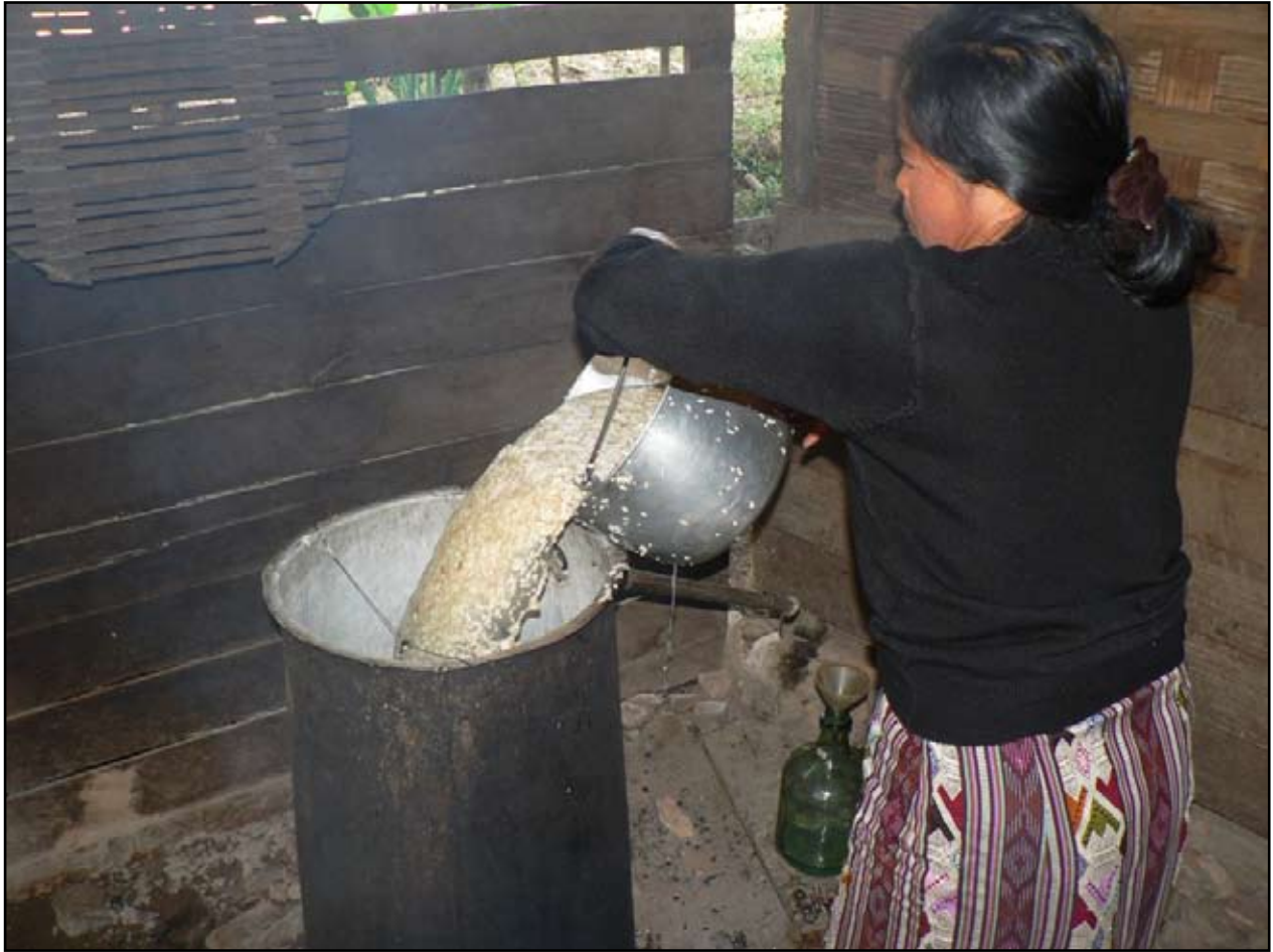
Figure 6. The process of distilling the rice starts - the fermented rice is poured into the mo .
