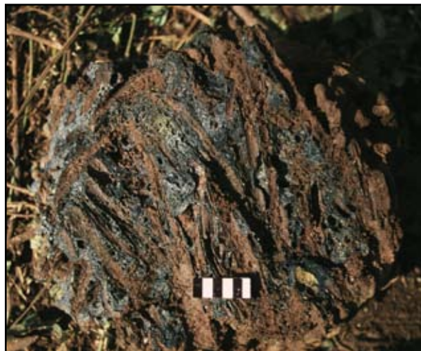
Figure 3. Plant impressions visible on a slag block from Kinanisi, Uganda (courtesy of A. Reid). Scale bar is graduated in cm.
