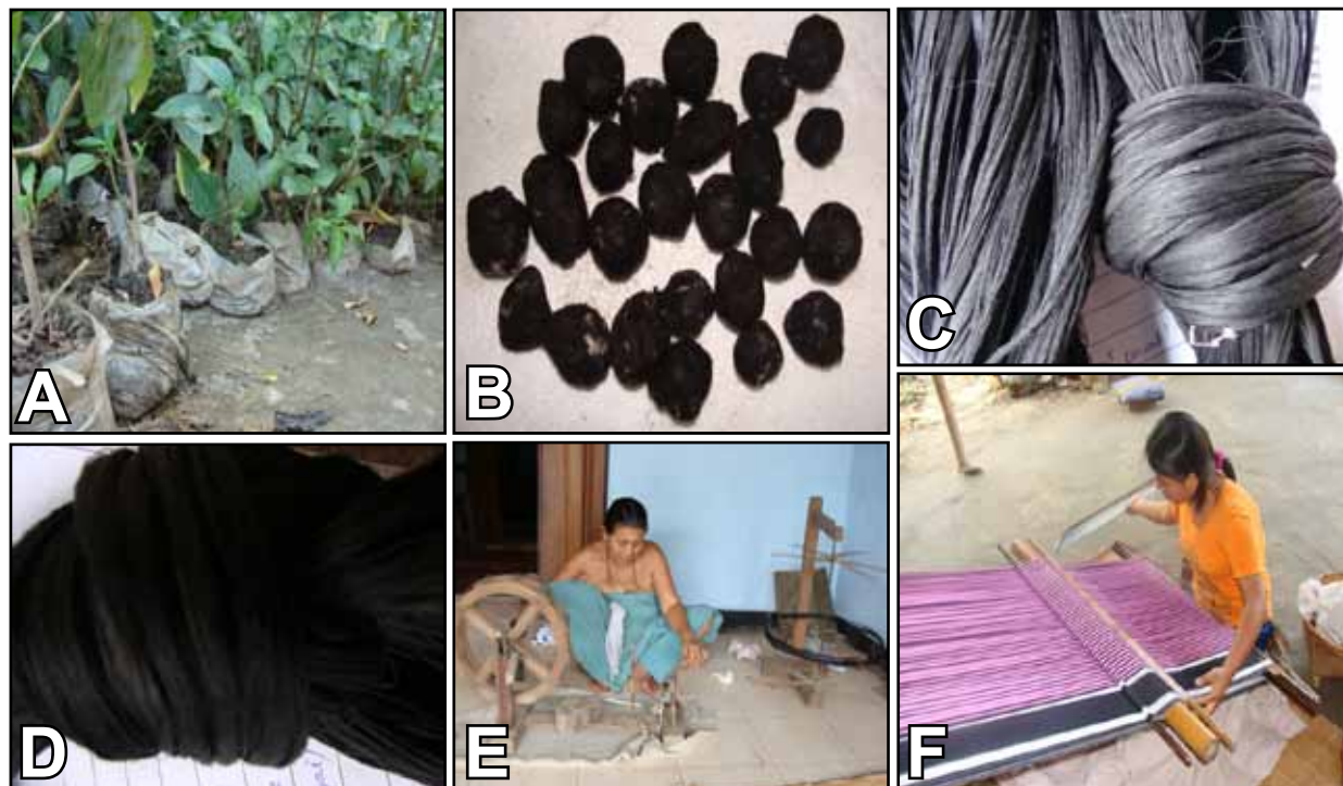
Figure 4. Process of kum dye production and yarn dyeing by Meitei community in Manipur, India. A. Strobilanthes cusia (Nees) Kuntze ( kum ) plantlets being vegetatively propagated; B. Kum cakes or paste; C. Chemical dyed yarn; D. Kum dyed yarn; E. Yarn preparation using the traditional instrument called tareng ; F. Weaving with a loin loom ( khwang ).
