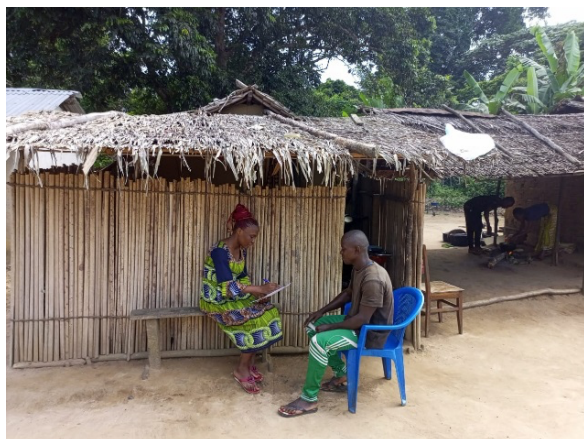
Photo 1: Palisade made of petioles of Raphia laurentii and roof covered with leaves of the same species.
