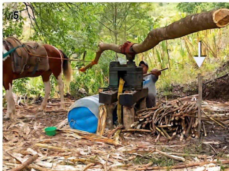
Figure 5. Trapiche . The arrow indicates a reference measure of 80 × 80 × 150 cm placed next to the trapiche , used to estimate the volume required to produce approximately 200 liters of cane juice.
