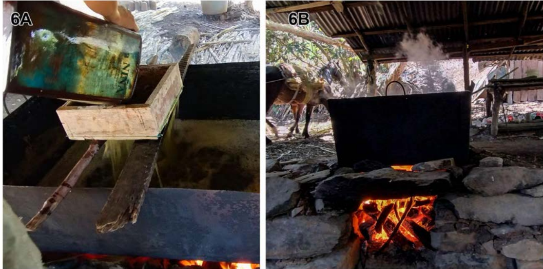
Figure 6. Cooking and reduction of the cane juice: (A) the extracted juice is filtered using a wooden colador and poured into the iron puntera ; (B) the puntera is placed over a wood-fired oven built with clay and stone for cooking.
