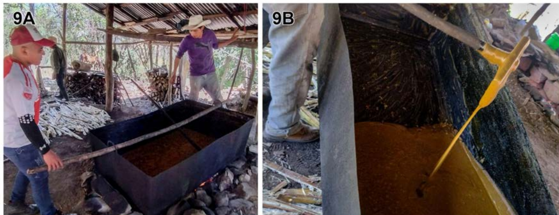
Figure 9. Solidification process: (A) the puntera is removed from fire with the aid of a long wooden pole to allow cooling; (B) with the help of the tool called rastrillo , the pilón is cooled for subsequent molding
