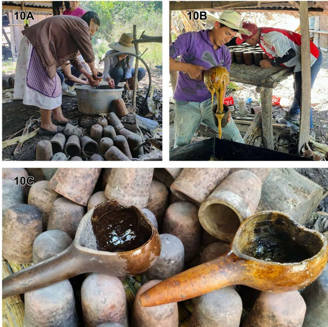
Figure 10. Molding of pilón : (A) clay molds are carefully washed; (B) pilón is poured into the molds with the aid of a guaje ( Lagenaria sp.); (C) guajes , the cucharón used to fill the molds with pilón .
