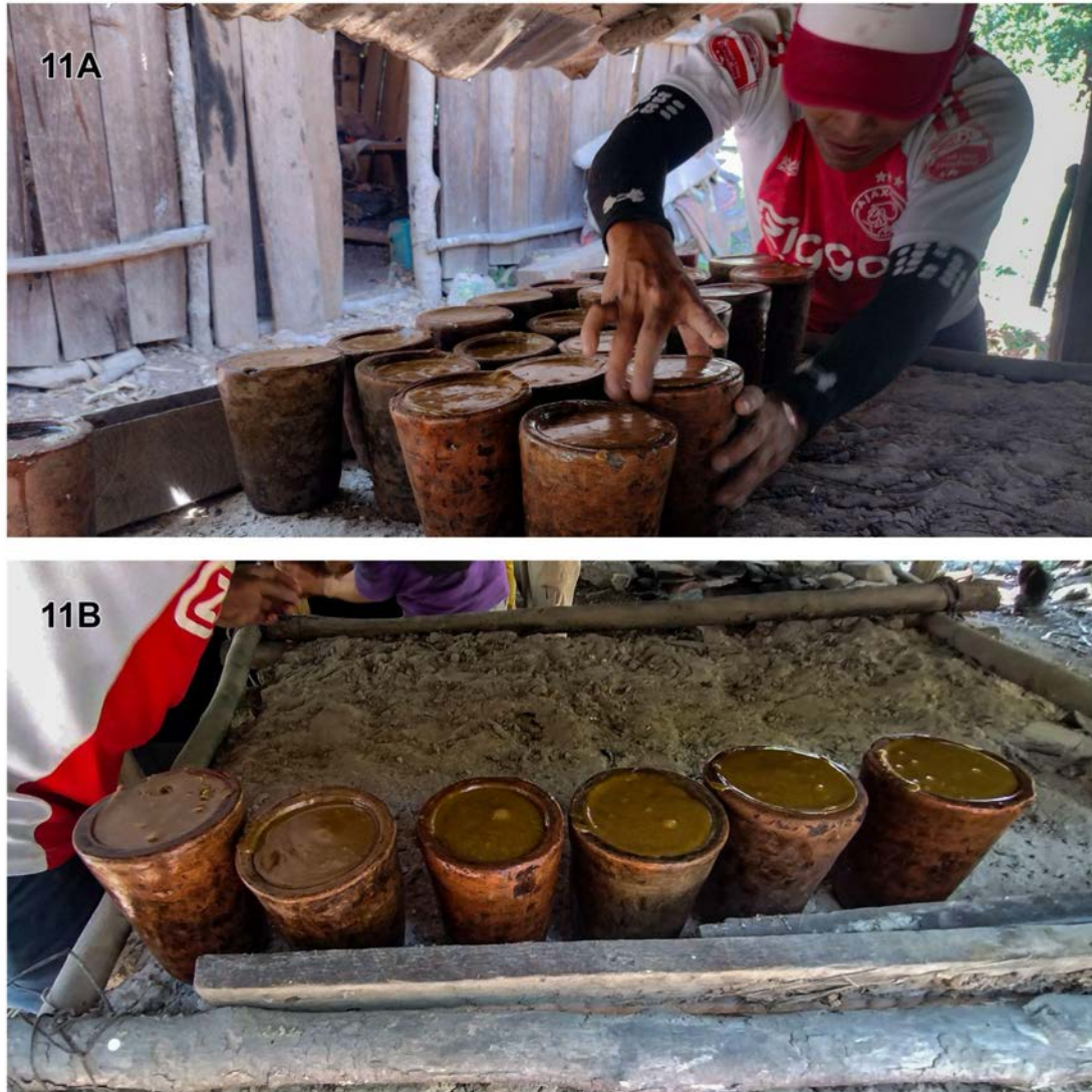
Figure 11. Arrangement of molds: (A) a group member arranges the freshly filled molds; (B) the filled molds are placed on a surface covered with fine ash, which ensures stability and facilitates cooling.
