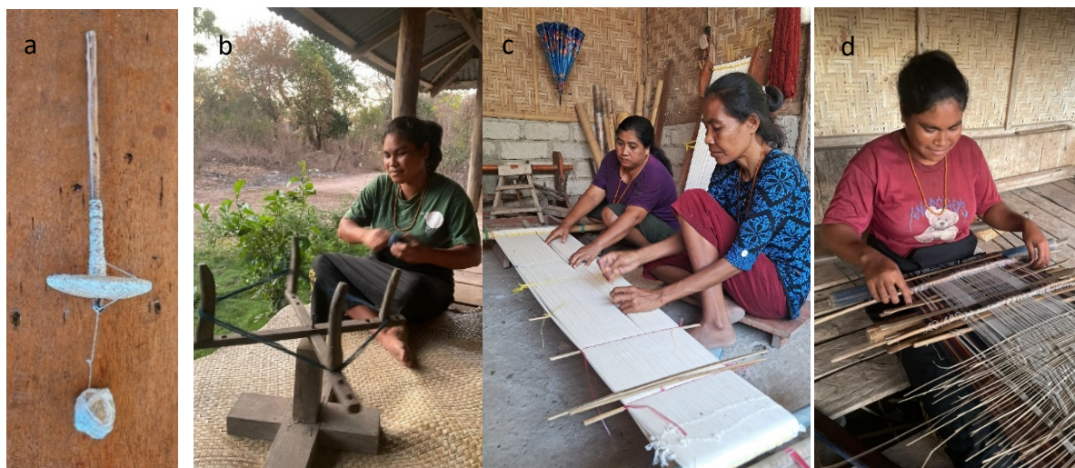
Figure 2. Traditional weaving tools of Sumba. (a) pahulur benang (cotton processing), (b) piepak (yarn winding), (c) wanggi kapala (warp arranging), (d) gedogan (loom). Source: Authors' documentation (2025). All photographs were taken with informed consent from the individuals depicted.
