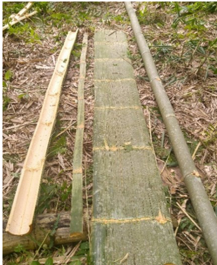
Figure 6. Components of traditional bamboo house (from left to right: lenga, lat, naja, tubo) in Ratogesa village.
