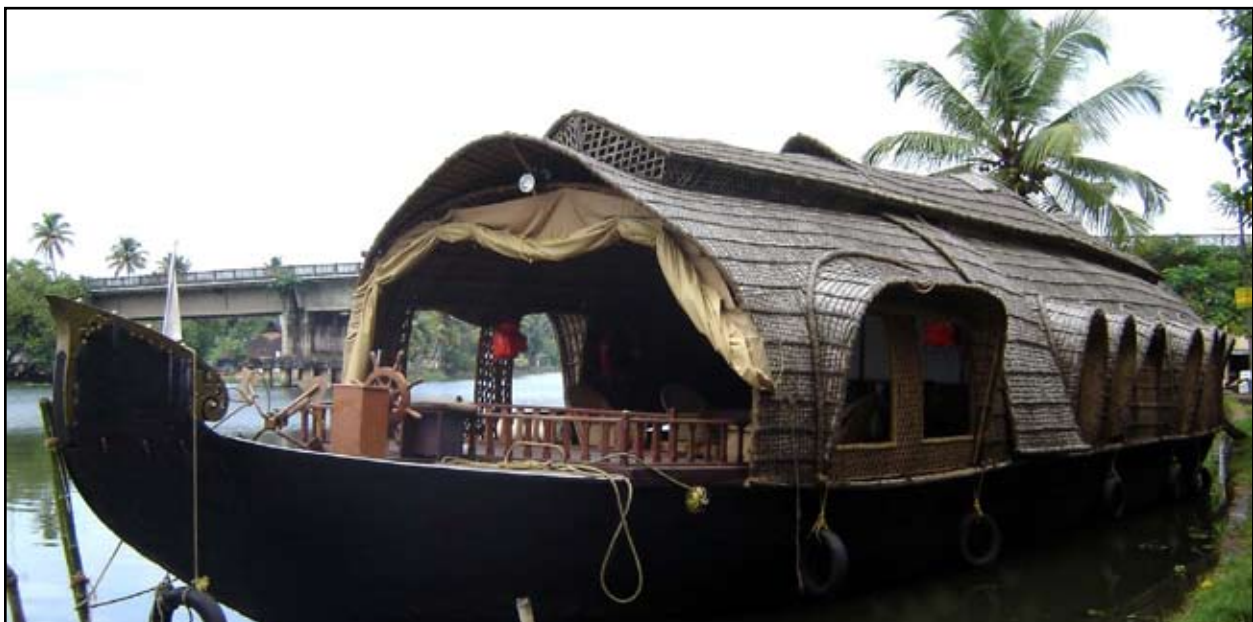
Figure 33. A luxury air-conditioned house boat made with a wild jack wood hull.
